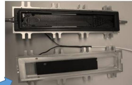
Advanced electrodes with high capacity of production of oxidants
