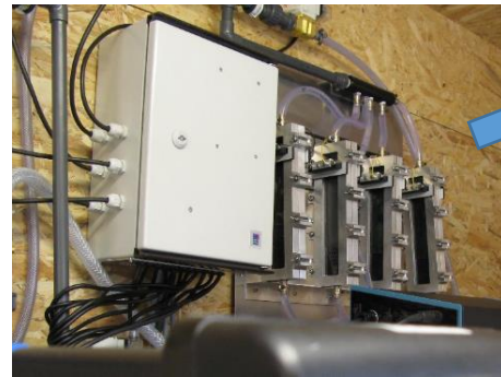
Electrochemical oxidation in electrolytic cell
